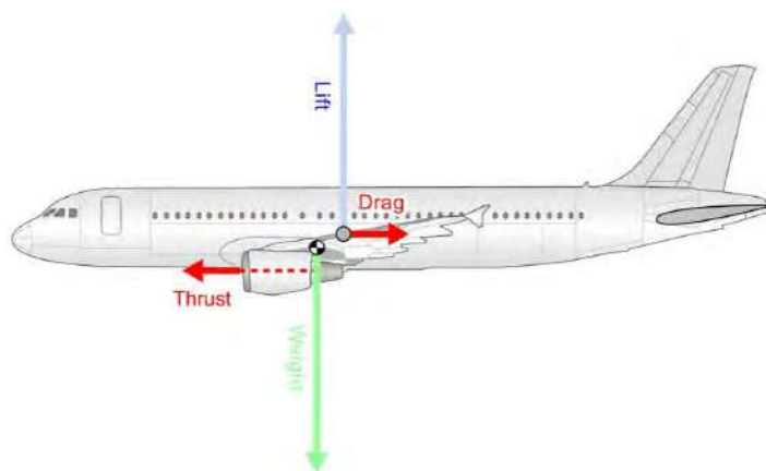
Figure 5.10 Typical force couples acting on an aircraft
