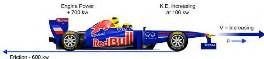
Figure 5.15 An excess of power over friction will lead to acceleration
