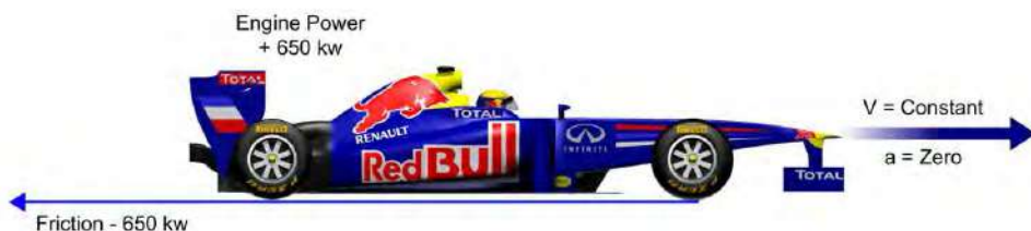
Figure 5.14 Energy out and in rebalanced - zero acceleration
