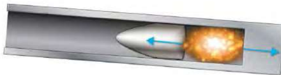
Figure 4.12 Equal and opposite forces are applied to both gun and bullet
