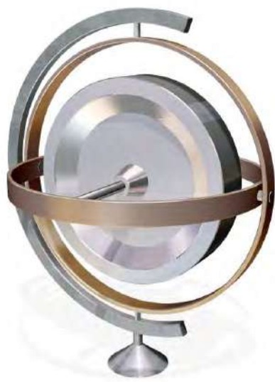
Figure 6.1 A typical gyroscope arrangement
