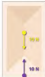
Figure 4.13 The equal and opposite forces acting on a brick
