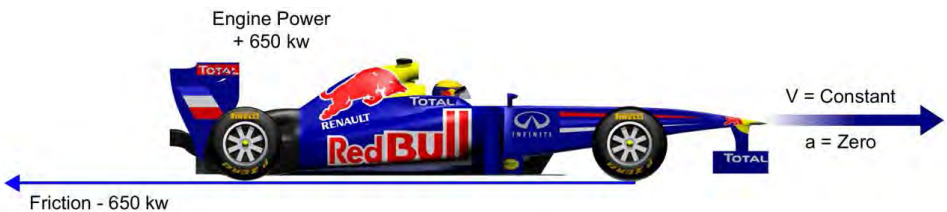
Figure 5.14 Energy out and in rebalanced - zero acceleration
