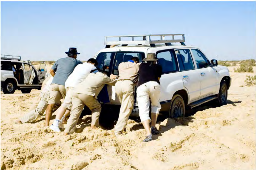
Figure 4.2 A continuous push is required to balance the frictional forces trying to slow the car
